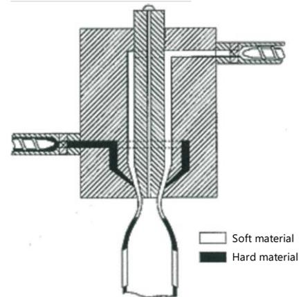
Fig. 1 Structure of Exchange Blow Molding and example of exchanged parison
