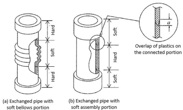
Fig. 2 Basic composition of Exchange - Blow molded part
