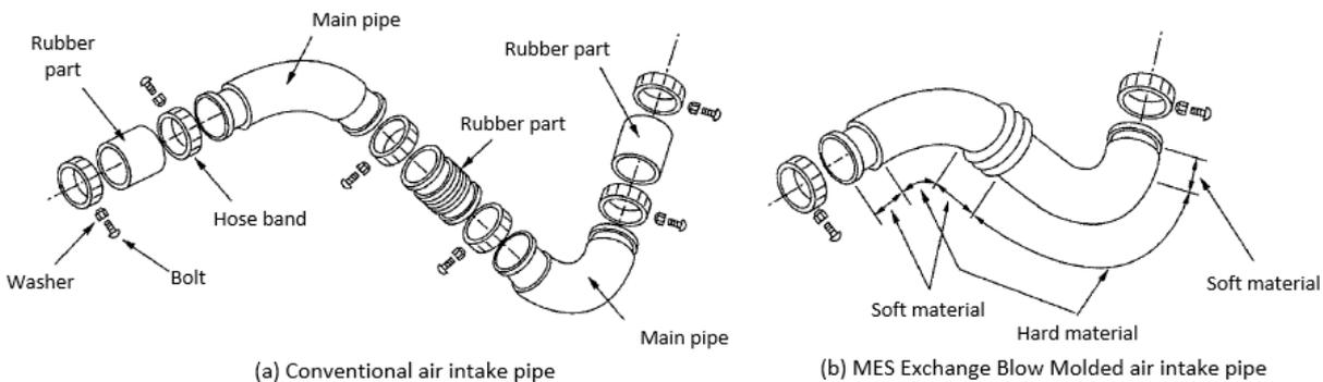
Fig. 4 Replacement of plastic in air intake pipe
