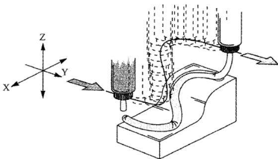
Fig. 3 Basic concept of MES (3D Blow molding)
