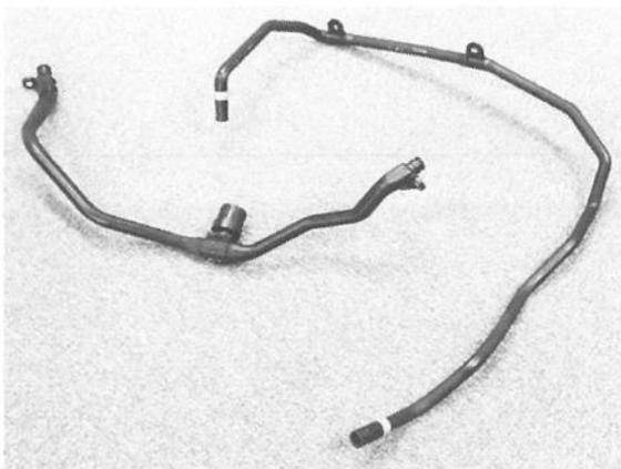
(Left) Main body: TPAE, Both ends: PA6  $\phi 18 \times L750$
